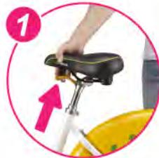
Press up the pull rod and adjust the saddle height.
